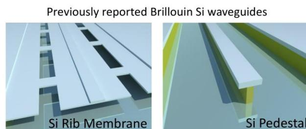
*Fig. 1: Schematic of previously reported Si Brillouin waveguides based on partial removal of the oxide cladding (left panel) and pedestal geometry (right panel).*
