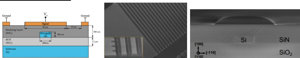
*Fig. 1: left: schematic view of a strained silicon waveguide. Middle: Grating coupler based on subwavelength structures. Right: SEM image of strained waveguide fabricated at C2N.*
