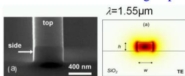
Fig. 1: Silicon wire waveguide
