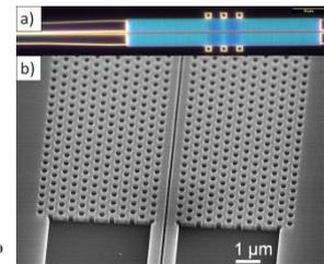
Fig. 3: Heterostructure photonic crystal cavity
